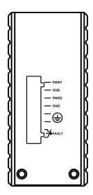
Field Wiring Terminal: Use Copper Conductors Only, 60/75°C, 12-24 AWG torque value 7 lb-in.
