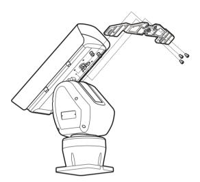
Connect the IR illuminators to the brackets. Lead the IR illuminator cable into the housing through the cable-clamps in the bracket and insert it in the housing through the cable-gland at the back of the housing.
