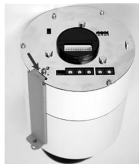
Attaching the wing to the Siqura MSD620
