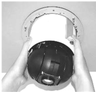
Securing the dome camera
