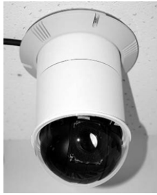
Hard-ceiling mounting (cables exposed)
