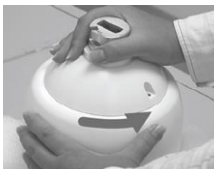
Figure 8a/b/c Remove the outdoor tube adaptor (left). Lubricate the optical cover's waterproof boot (centre). Attach the optical cover to the dome body (right).
