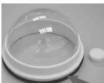
Figure 8a/b/c Remove the outdoor tube adaptor (left). Lubricate the optical cover's waterproof boot (centre). Attach the optical cover to the dome body (right).
