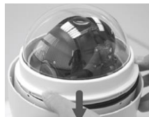
Figure 8a/b/c Remove the outdoor tube adaptor (left). Lubricate the optical cover's waterproof boot (centre). Attach the optical cover to the dome body (right).
