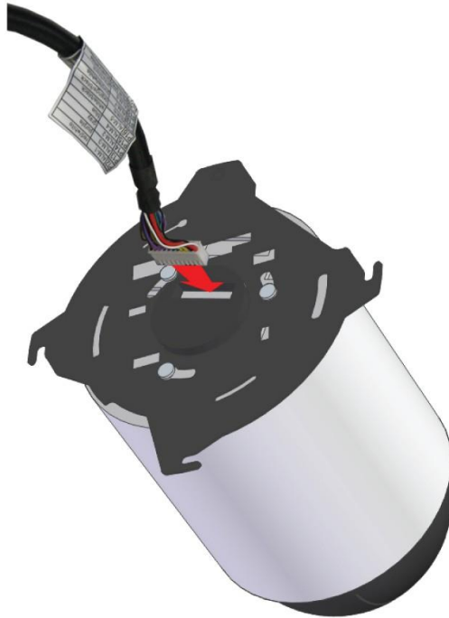
Attaching cable to the pressurized camera
