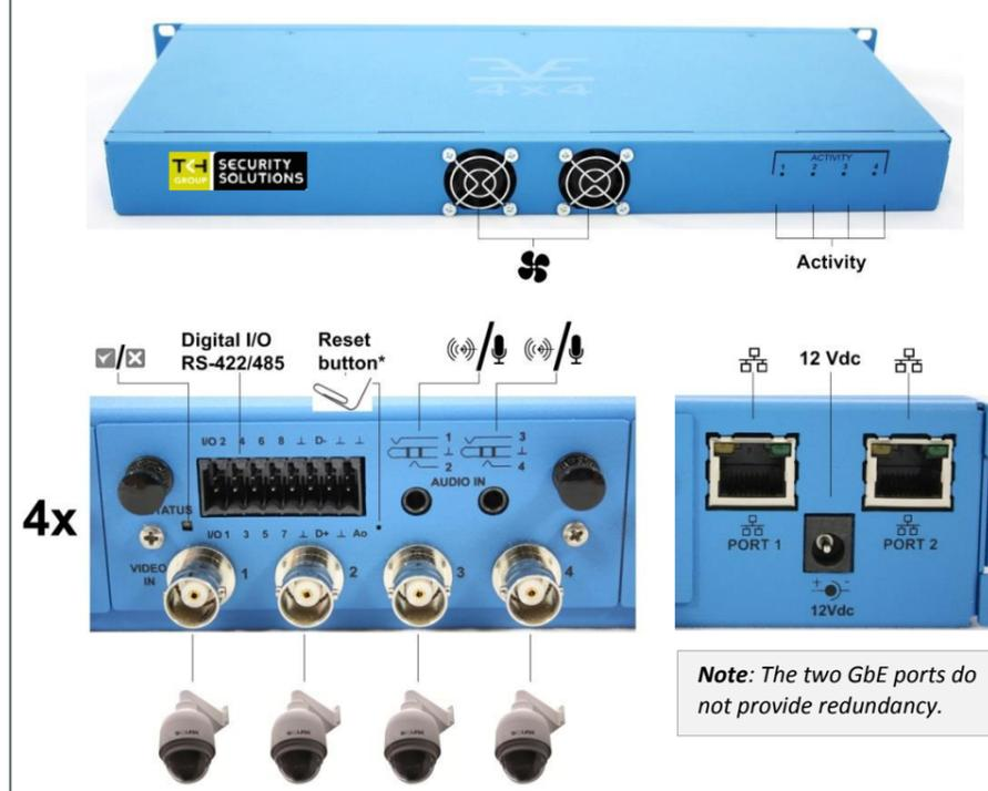
*Note: The two GbE ports do not provide redundancy.*
