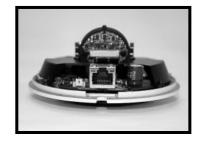
Connect one end of the Ethernet cable to the RJ-45 connector of the indoor camera, and plug the other end into a PoE switch.
