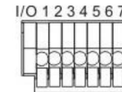
Figure 3 Diagram of Alarm I/O and RS-485 connection pins
