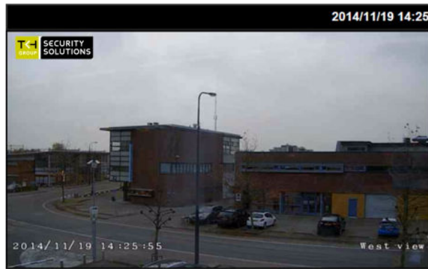
Camera view with three overlays: Image overlay (top left), Date & time (bottom left), and Text string (bottom right)
